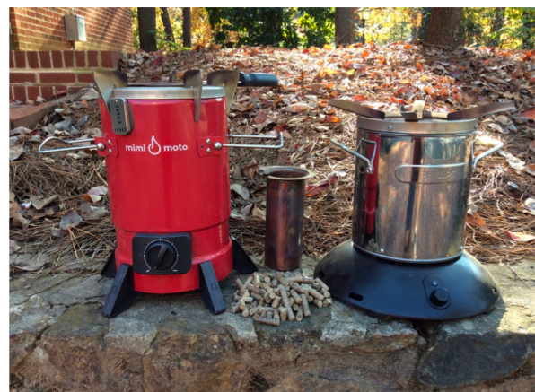
Figure 2: Micro-gasification cookstoves used by Inyenyeri.. These stoves are clean-burning and use biomass fuel pellets. Image from [6].
